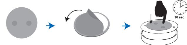
**c** Assembling the smoke alarm to the ceiling: The base of the smoke alarm is simply placed against the ceiling element. To remove the smoke alarm, do not pull down vertically but slide it sideways of the ceiling element.
